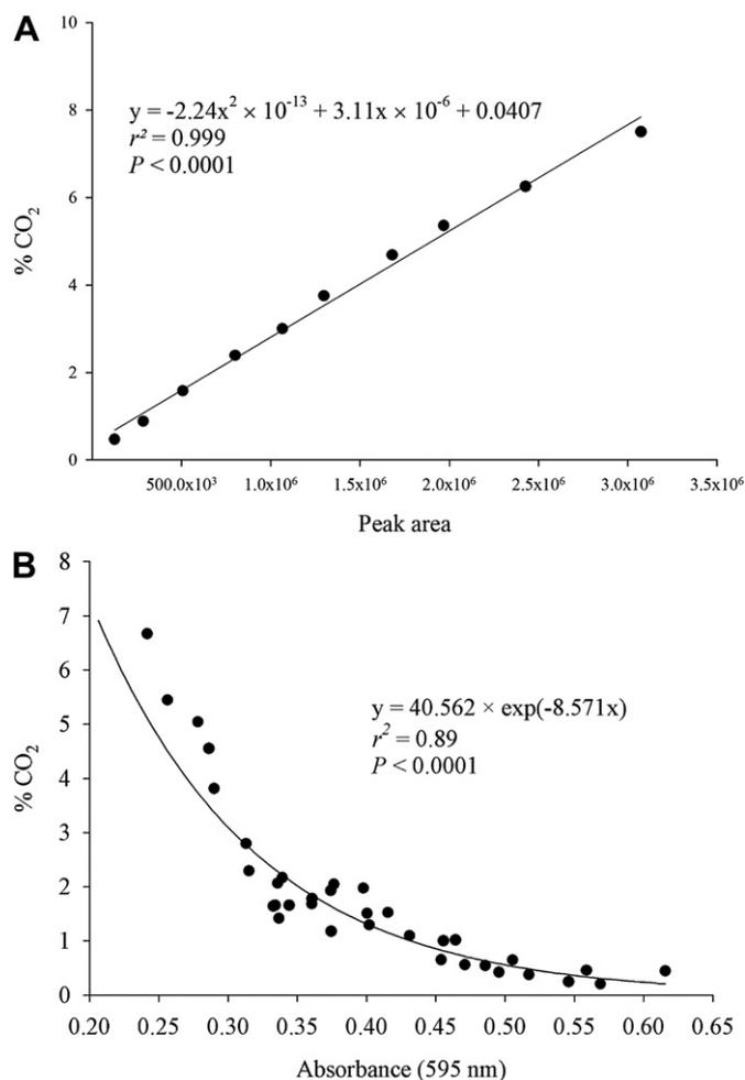
**Fig. 1.** Calibration of the color change experienced by the indicator solution with the gas chromatograph. A) Relationship between the peak area and the concentration of the standard CO<sub>2</sub> (n = 10). B) Calibration curve for absorbance vs. percentage of CO<sub>2</sub> (n = 36).
